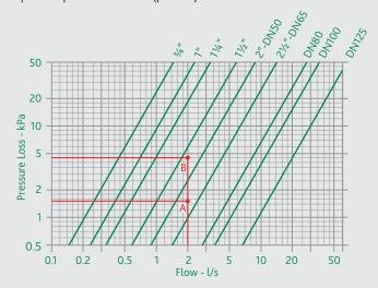
Using the 610 series flow chart, with a flow rate of 2 l/s, moving up vertically the A and B points are identified, which are obtained at the intersection with the respective pressure loss values.
