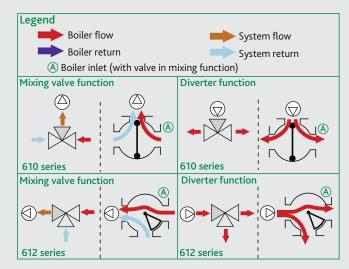
Typical installation of 610 series 3-way butterfly with mixing function
