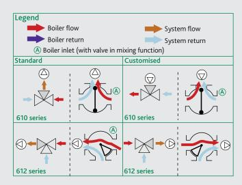
Typical installation of 612 series 3-way sector with mixing function
